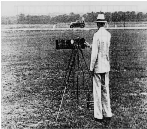
Fig. 2: Greenshields measurement set up for the reported 75 years ago
