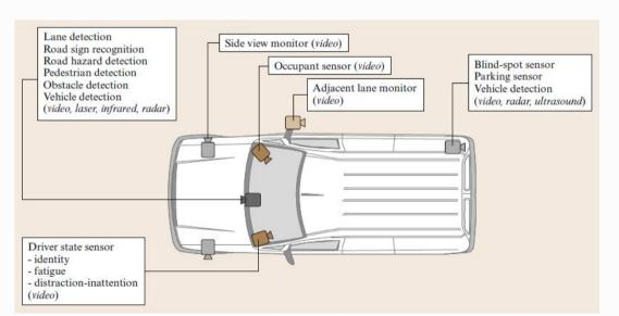
Radar is generally used for obstacle detection at a distance, while infrared and ultrasound are used for close proximity obstacle detection. Laser ranging and image processing are used to more robustly recognize the road scene under various weather conditions.
